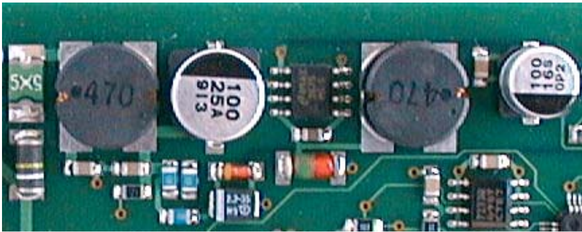
Figure 15.6: The PTC-IIpro switch-mode power unit.
