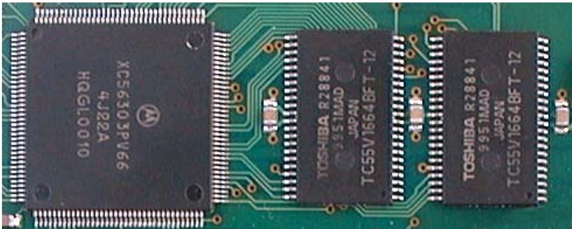
Figure 15.5: All digital, the signal processor with RAM
