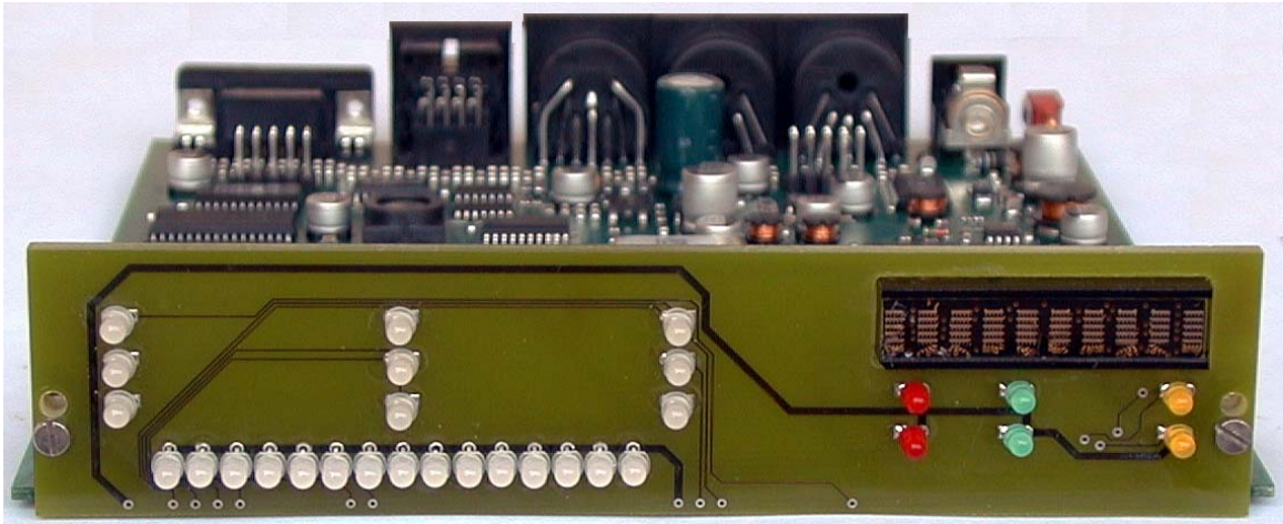
Figure 4.2: The PTC-IIpro front panel
