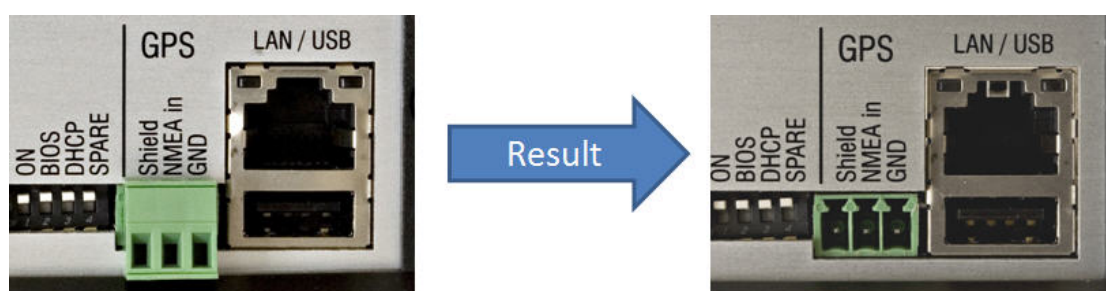
Figure 2: Removing the screw terminal, example shows DR-7800
